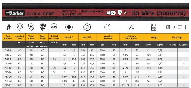
Reinforcement: Two-braid steel wire for sizes -4 to -6 | Four- or six-compact spiral steel wires for sizes -8 to -32
