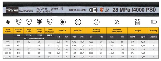
Reinforcement: Four-spiral steel wire
