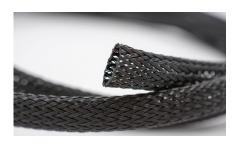
Tufftex M is a highly expandable and flexible sleeve manufactured from durable polyester filaments. Ideal for bundling lines and protecting from abrasion in automotive, appliance, industrial, and consumer applications due to the abrasion resistance and ease of use. The convenient braided construction allows for expansion over fittings, easy installation over long lengths, and the ability to conform neatly to tight bends.
