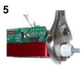
5.- Put the liquid tight fitting back and tighten
