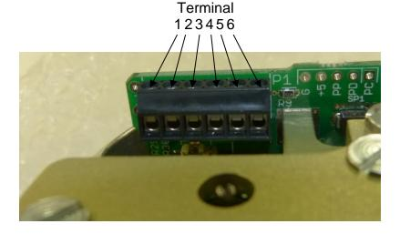
Locate the correct connection terminals as shown in the picture to the left then connect according to the connection schematics above.
