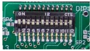
DIP switches. In this example DIPs 1, 2, 6 and 12 are on.
