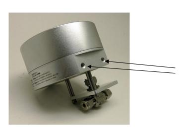
Holes for a mounting bracket. Holes are threaded for ¼-20 and are approximately .275" deep.
