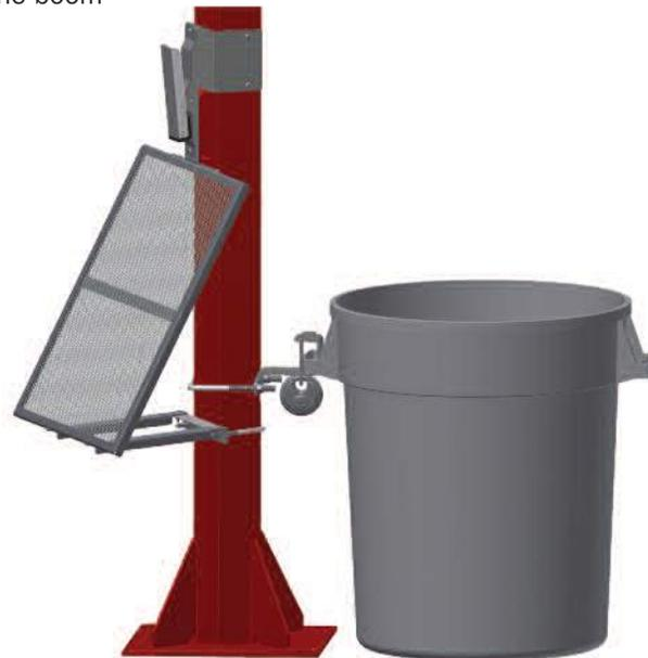
OPTIONAL MODULAR MAT RACK ASSEMBLY (75000-111A) AND OPTIONAL TRASH CAN ASSEMBLY (75000-114A)
