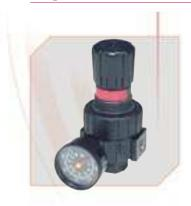
Using a unique rolling diaphragm design with no wear points, Alemite Regulators are constructed to ensure a longer service life than standard flat diaphragms. Capable of reverse flow and repeatable performance, these regulators provide accurate regulation over a wide range of pressures, even in the most demanding industrial applications.
