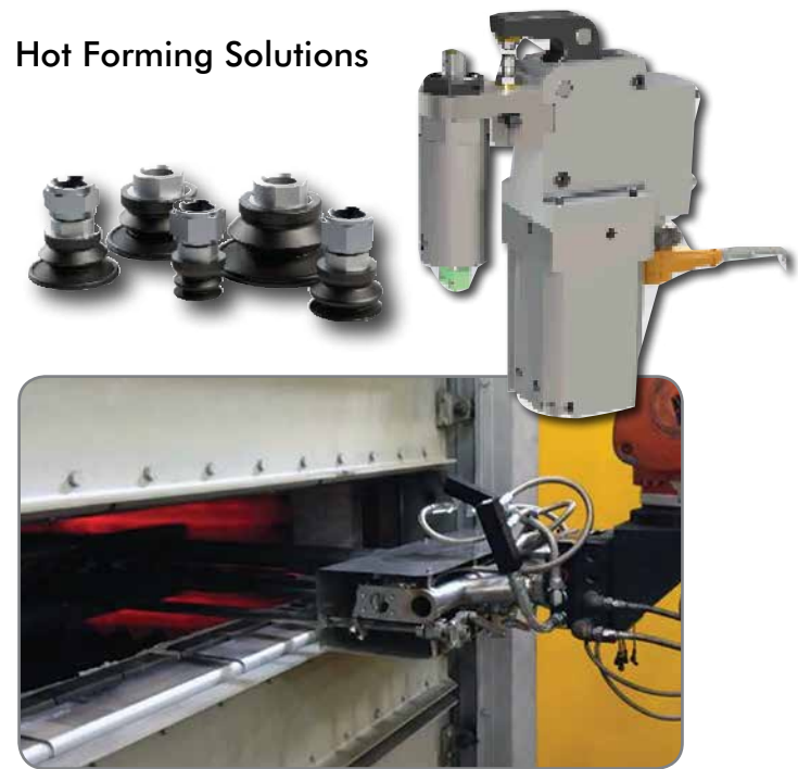
40mm/1.50" Receiver with Air and Electric Connection
