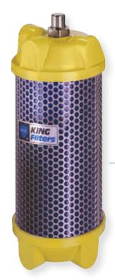
**KING Visi-Guard 1716 Dryer** utilizes a desiccant bed to remove water or oil vapor for critical compressed air needs. (Choice of desiccant media selection determines application.) The Visi-Guard acrylic chamber is especially suited for SG-1 indicating silica gel that changes from blue to pink when the air supply approaches 20% RH. Properly maintained, the dryer can reduce dew point to -50°F/-45°C. (Alternate AC-1 desiccant can reduce oil vapor content to less than 0.5 PPM w/w.)
