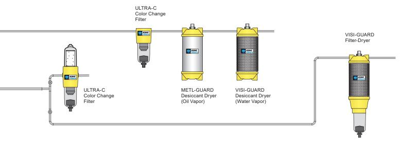
replacement. A combination filter-regulator-gauge comprises the Ultra-C Air Control Station. Each is offered with an automatic drain sump to reduce maintenance and assure continuous dry compressed air.
