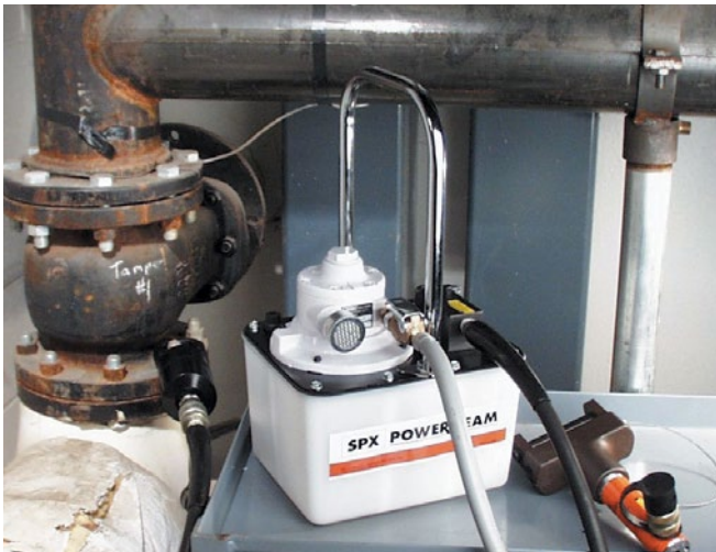
▶ The PA17 used with a flange spreader
