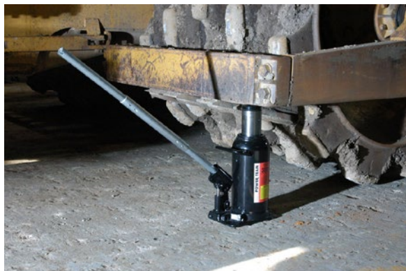
9130A Low Profile Hydraulic Bottle Jack provides the lifting capacity and low height for this underground mining application.
