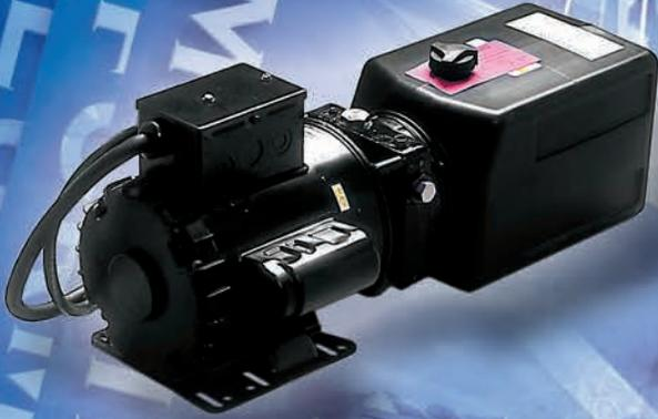
This power unit is designed for smaller, low-rise auto hoists and can be mounted either horizontally or vertically, operating on AC power. A push button on the motor starts the unit to raise the vehicle on the lift. To lower, a manually operated cartridge-style release valve is used for finger-tip control of lowering speed.
