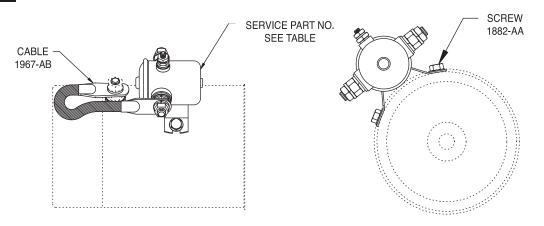
**Figure 1 Internal Ground**
