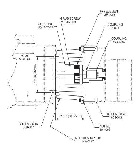
Suitable for use with IEC 90 Frame motors with an 95C (B14) interface and a 24mm diameter shaft, measuring 50mm long from mounting face.
