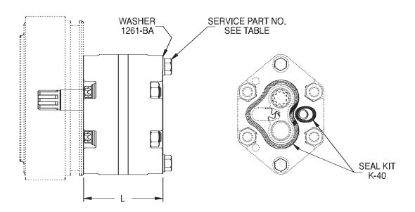
Current Endhead Design Uses 5/16-24 Mounting Thread. Older Endhead Design Used M8 Mounting Thread. Pump Kits Include Both Imperial And Metric Mounting Bolts.
