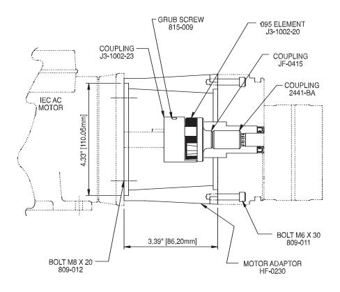
Suitable for use with IEC 100 frame motors with an 110C (B14) interface and a 28mm diameter shaft, measuring 60mm long from mounting face.
