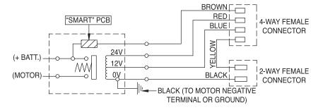
Rated for use up to 300 amps (intermittent), completely sealed construction eliminates need for circuit breakers, fuses or microswitches, dual voltage– 12 and 24 VDC, non-weldable contacts, interchangeable with current designs, neat one-plug wiring harness, terminals can not be over-tightened, covers single and double terminal applications, waterproofed to IP67, electronics suitable for use in ambient temperatures between -40° F(-40° C) and 185° F (86° C), world patents applied for.
