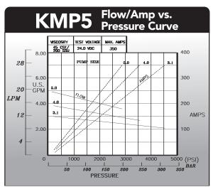
For flows over 3 U.S. GPM (11 LPM) use 1413-AA filter
