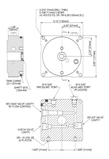
Endhead cannot be used with manifold valves.
