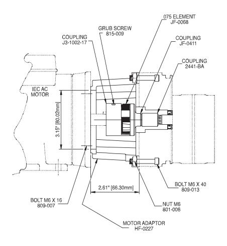
Suitable for use with IEC 80 Frame motors with an 80C (B14) interface and a 19mm diameter shaft, measuring 40mm long from mounting face.
