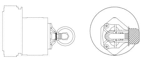
Parts may be assembled in either orientation depending on mounting of power unit. For flows over 3 GPM use 1413-AA large filter.
