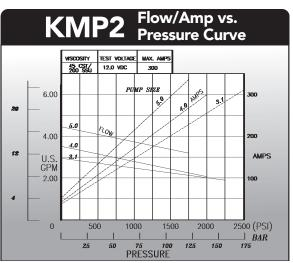
For flows over 3 U.S. GPM (11 LPM) use 1413-AA filter
