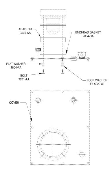
For use with KR71 and KR73 tanks to give additional clearance for valve coil.
