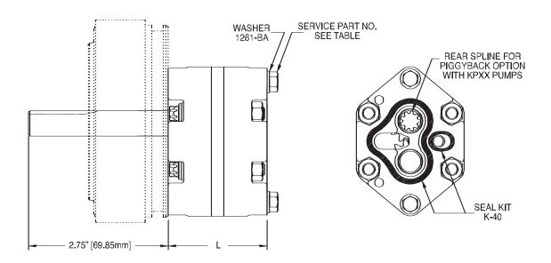
Current Endhead Design Uses 5/16-24 Mounting Thread. Older Endhead Design Used M8 Mounting Thread. Pump Kits Include Both Imperial And Metric Mounting Bolts.
