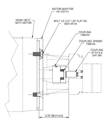
Mount H2-1007-01 to motor before assembling to KM97.
