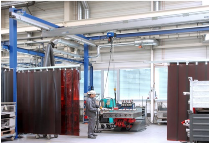
Aluminum single bridge crane system with reinforced section and a conductor line used with a chain hoist and a magnet
