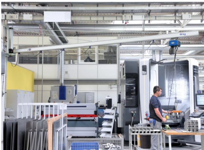
Aluminum wall mounted jib crane with chain hoist and magnet during loading of a milling machine
