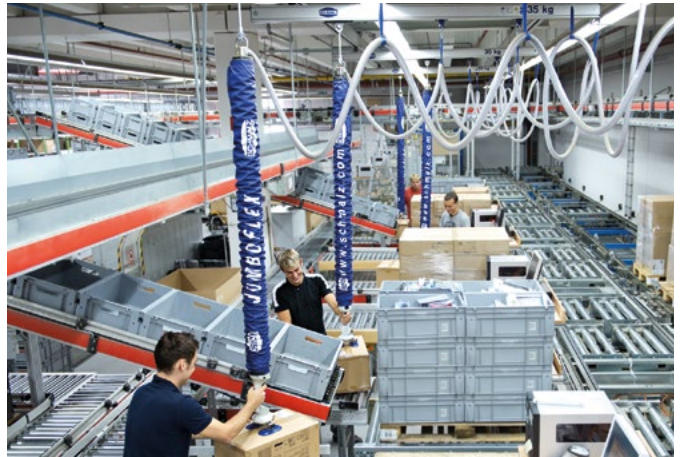
Aluminum multi bridge crane system with vacuum tube lifters JumboFlex commissioning packages
