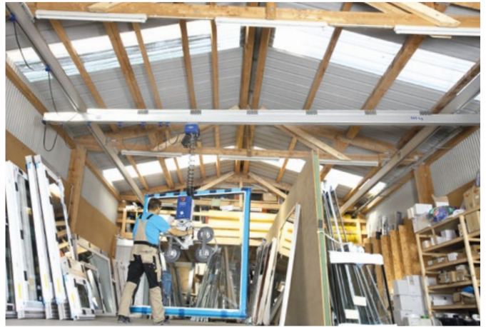
Aluminum single bridge crane system with reinforced section and vacuum lifting device VacuMaster Window during handling of windows
