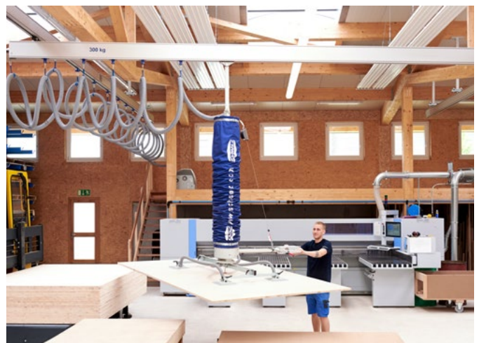
Aluminum single bridge crane system with vacuum tube lifter JumboErgo loading a CNC machine
