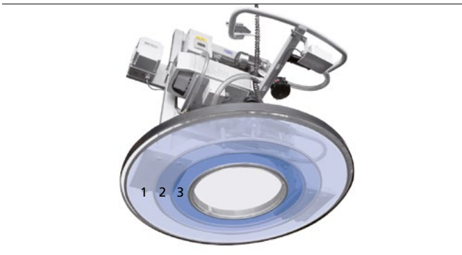
Suction plate with three separate vacuum clamps
