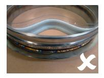
All care must be taken to ensure that the circumference of the head after fitting and welding remains the same size as supplied, to ensure fitting tolerance of the connector.
