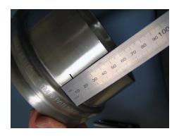
Avoid cutting the tail down if possible. If it is necessary to shorten it, we recommend leaving at least 15mm (1\%2") on the tail.
