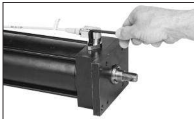
Bolt sensor to cylinder.
