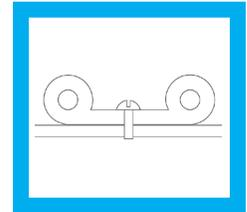
**Press Fit into Notch:** When properly designed, the "notch" method can eliminate the need for adhesive, additional hardware and groove. Primarily utilized as door
