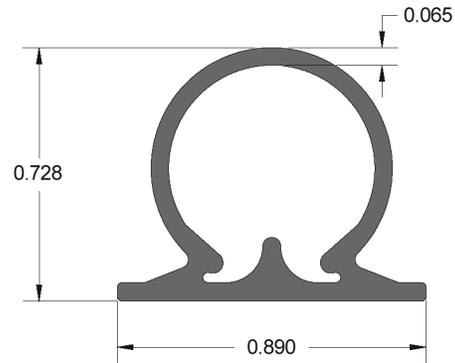
Figure 7 - Simple Drawing of Omega Profile
