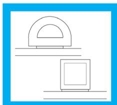
**Hardware Captured:** This attachment method typically does not require adhesive to hold the seal in place nor a groove, while assuring capture of the seal by utilizing hardware.
