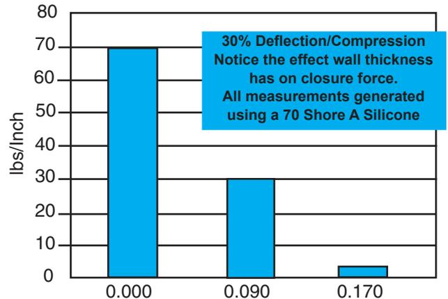
**Figure 6 - Effect of geometry on closure force**
