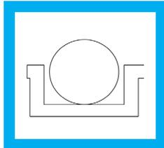
**Groove for Friction-Fit Seal:** Only possible with Hollow-O cross-sections or special custom designed profiles. Not possible with Solid-O's due to gland overfill concerns. Groove walls provide compression stop. TechSeal Friction-Fit Seal Designs aide in assembly without using adhesive.
