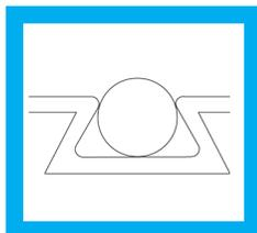
**PSA Backed Extrusions:** Provides "No-Groove" Sealing. Good solution for low pressure sealing of enclosures where machined or cast grooves are not practical due to thin covers. Typically utilized as outdoor environmental seals capable of passing wind driven rain tests.
