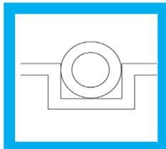
**Dovetail Groove:** Commonly used groove type for molded or spliced o-rings in vacuum sealing. Dovetail groove holds the seal in place in such a way where it cannot fall out while allowing area in the corners for the seal to move under compression. These grooves are very expensive to machine, and the tolerances are especially critical. Therefore, it should be used only when it is necessary.
