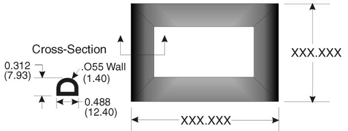
**Figure 2 - Typical TechSeal Picture Frame Gasket**
