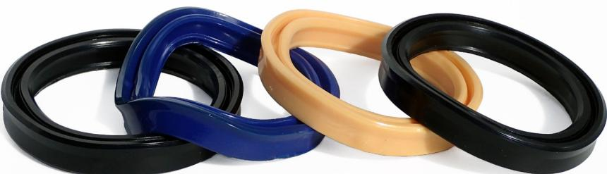
Polyurethanes are a thermoplastic elastomer. High heat causes the material to soften. High heat melt sample of Resilon 4350 seals (black), Resilon 4300 seal (tan), Leading competitor seal (blue) shown above.
