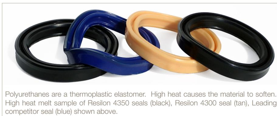
Polyurethanes are a thermoplastic elastomer. High heat causes the material to soften. High heat melt sample of Resilon 4350 seals (black), Resilon 4300 seal (tan), Leading competitor seal (blue) shown above.
