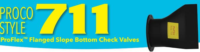
The **Proco Style 711 ProFlex™** check valves are engineered for installation on pre-existing pipe lines such as manholes, outfalls, vaults, where the outfall invert of the pipe is close to the floor of the manhole or outfall. When a new installation is being designed, the 711 valves can be engineered into the pipe layout with little concern for outfall clearance due to its "low slope" design.
