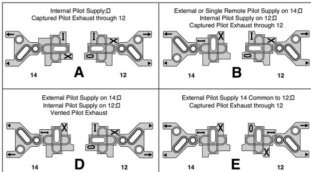
\* PJLP02 Manifolds can be used for External Pilot, **NOT** Remote Pilot
