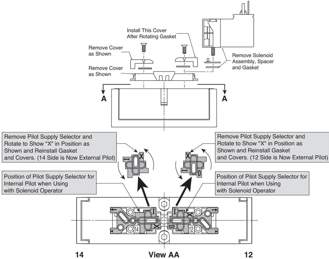
**Changing from External Pilot Supply, Vented Pilot Exhaust to Internal Pilot Supply, Captured Pilot Exhaust**
