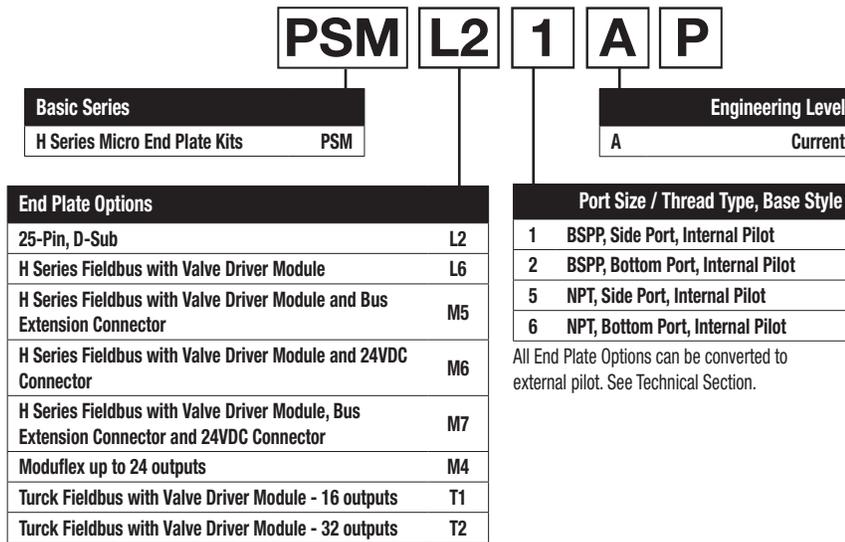
All End Plate Options can be converted to external pilot. See Technical Section.
