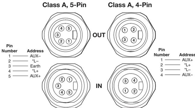
\* 7/8" logic power has no connection to internal P2H unit but does carryover to OUT 7/8" connector (for jumper logic power only). Logic power for P2H unit will be supplied from M12 (pin 1 & 3).
