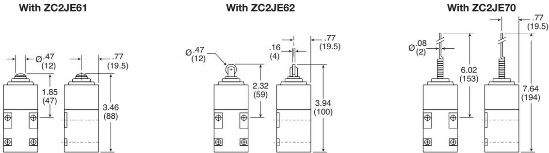
**Switch Body With Rotary Heads and Operating Levers**
