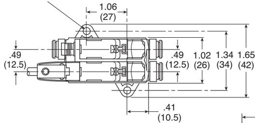
Surface Mounting with Screws 4 mm Dia. into Retractable Brackets 3mm Thick
