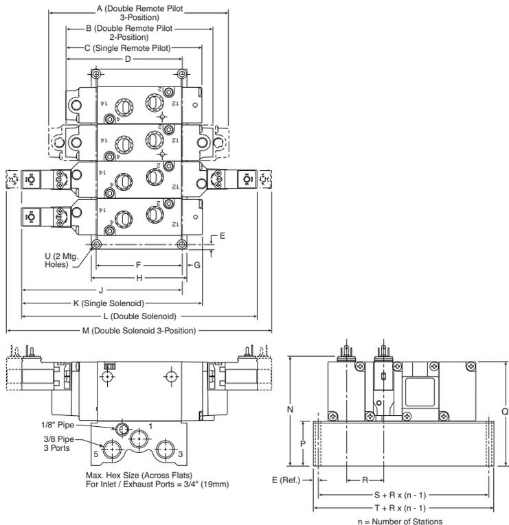
**B5 4-Way IEM Aluminum Bar Manifold**
