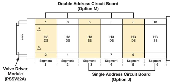
**HB, HA, H1, H2 - Nine Segment Manifold with Intermediate Supply Example**
