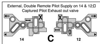
**DX01 Manifold Assembly Schematic for External Double Remote Pilot Selector Gasket Position C**
