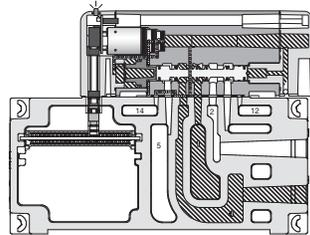
**15407-2** 18mm Single Solenoid Internal Pilot Manifold Mounted
