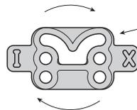
Remove Gasket and Rotate to Show "I" in Position as Shown and Reinstall Gasket and Covers. (Valve is Now External Pilot)
