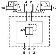
**H2 Common Port Regulator Shown - Double Solenoid, 14 Energized, Internal Pilot**
