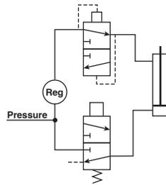
**Dual Pressure Actuation of Double Acting Cylinder**
