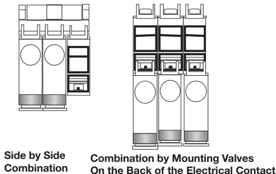
**Assembling Output Devices and Heads On ZB5 Series Mounting Block**
