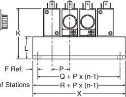
**P2LBZ 3/2 Single & Double Operators – Solenoid & Remote Air Pilot**
