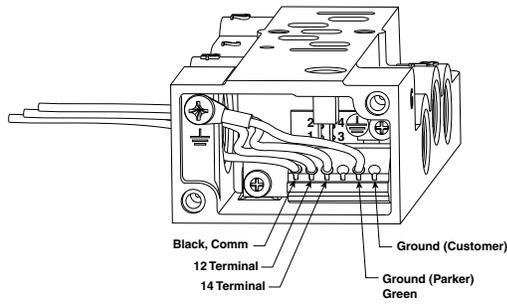
All commons internally connected on terminal strip
