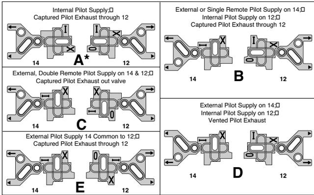
**DX02 & DX01 Subbase Assembly Schematic for Captured Selector Gasket Positions A, B, C, D and E**
