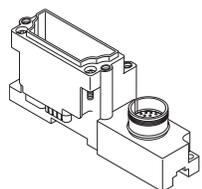
BL67 base modules are aligned one by one to the right of the communication module and are tightened each with two screws, either with the communication modules or with the previous module. A DIN rail is not required. This way a compact and stable unit is created which can be mounted directly on the machine.
