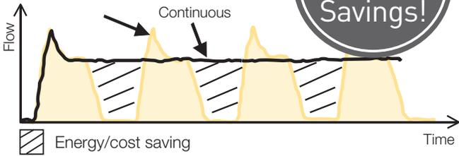
When using an Air Saver Unit several significant benefits can be achieved. Air blowing accounts for almost 50% of all compressed air used in plants. By using switching valve technology the Air Saver Unit can reduce air consumption by up to 50%!
