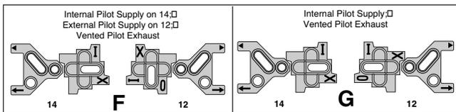
**DX02 & DX01 Subbase Assembly Schematic for Vented Selector Gasket Positions F and G**
