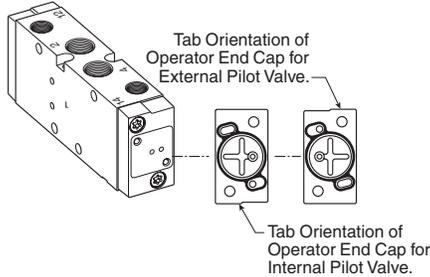
The 12 & 14-Ports are always tapped no matter what Valve Type / Function is selected. For Internal Pilot Function, ports do NOT need to be plugged.
