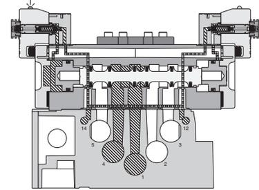
**H3 5599-2** Double Solenoid External Pilot Subbase Mounted
