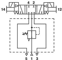
**H2 Common Port Regulator Shown - Double Solenoid, 14 Energized, Internal Pilot**
