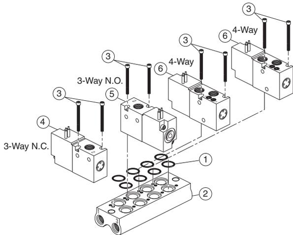
**Subbase Valve and Manifold Assembly**
