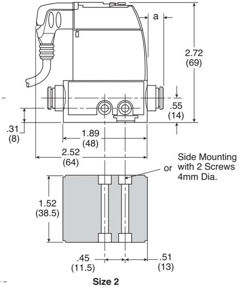
Side Mounting with 2 Screws 4mm Dia.
