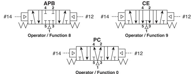
**With #12 operator signaled** – inlet port 1 connected to cylinder port 2, cylinder port 4 connected to exhaust port 5.
