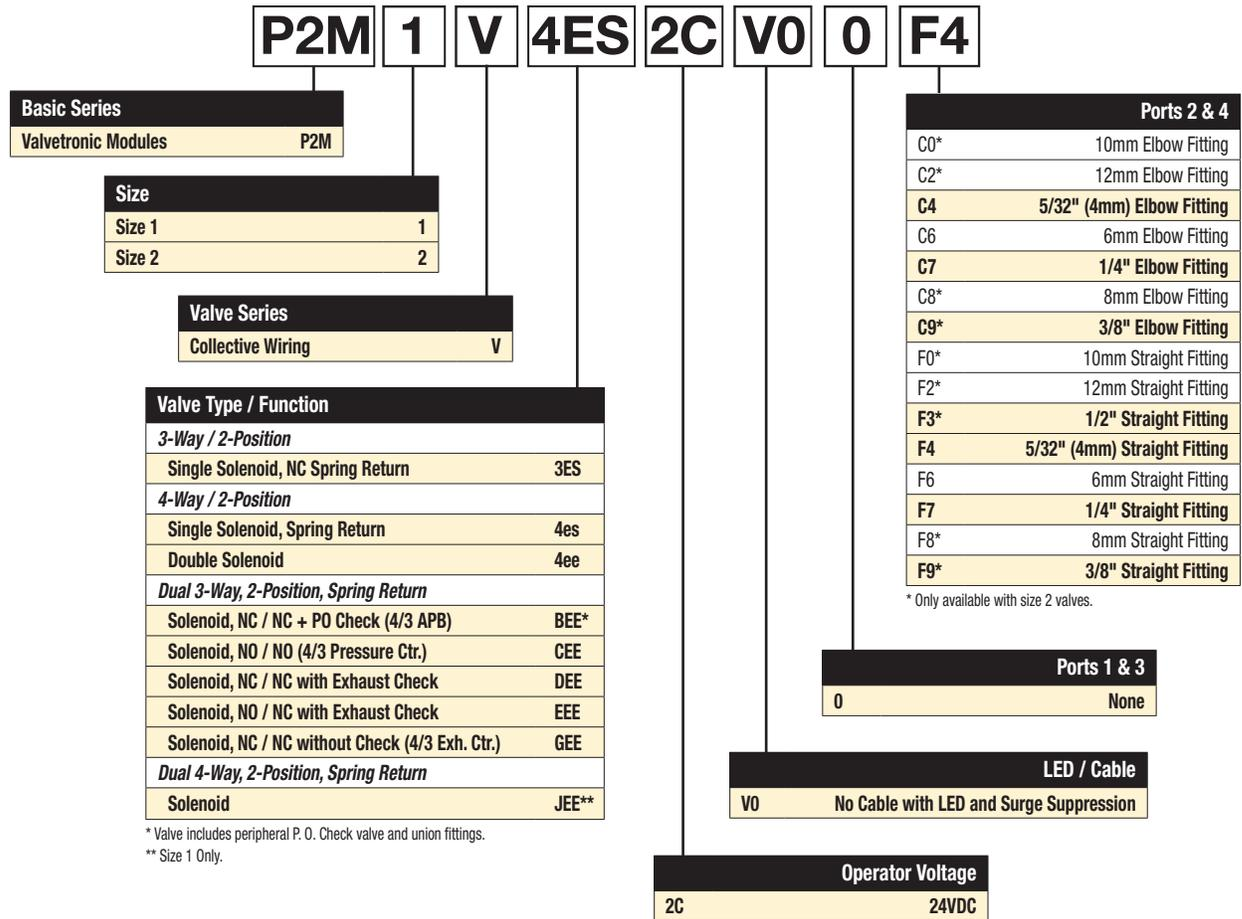
\* Valve includes peripheral P. O. Check valve and union fittings.
