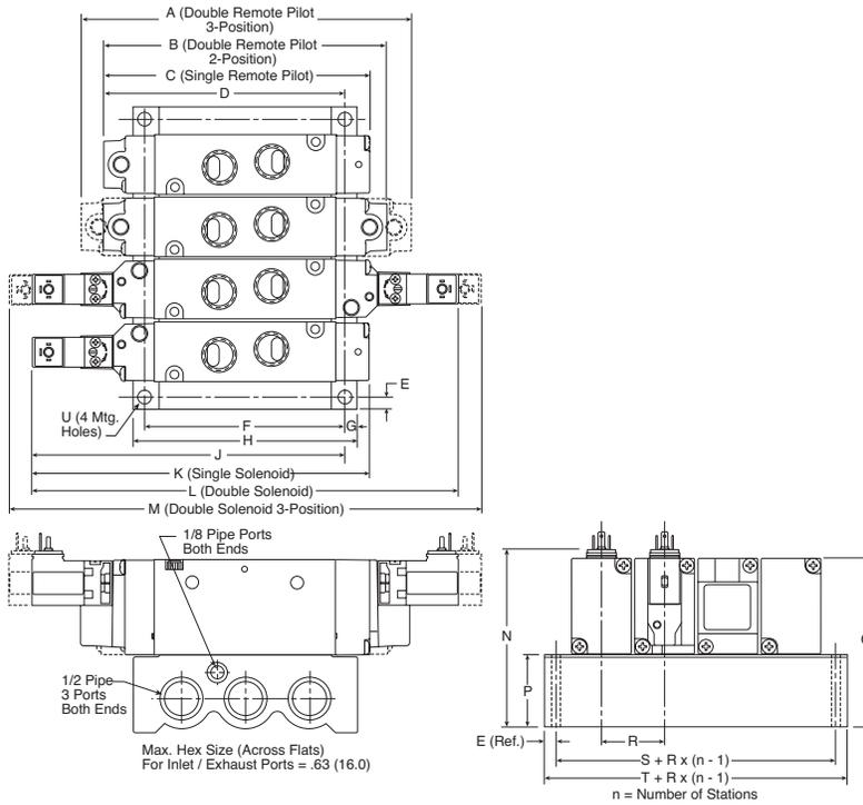
**B6 4-Way IEM Aluminum Bar Manifold**
