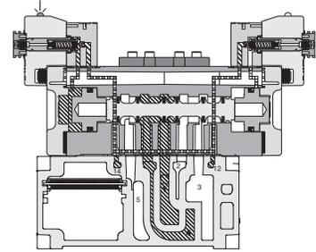
**H2 5599-2** Double Solenoid External Pilot Manifold Mounted
