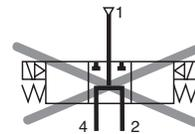
A traditional 5/3 pressure center valve is now replaced by a double 3/2 NO+NO valve module. The function is identical.
