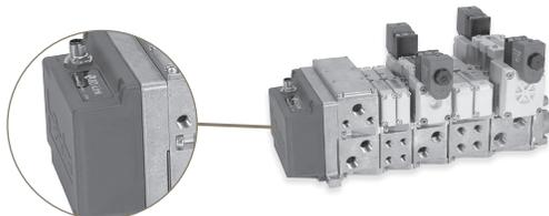
The Class B node has (1) 5 pin M12 connector to connect IO-Link for communication to a Class B IO-Link master, logic power and auxiliary power for the valve solenoids (up to the limit of the Class B node output\*).
