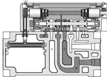
**15407-2** 26mm Double Solenoid External Pilot Manifold Mounted
