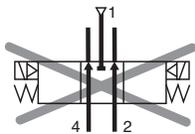
A traditional 5/3 center exhaust valve is now replaced by a double 3/2 NC+NC valve module (version with no exhaust check valves). Both cylinder chambers are exhausted and rod and piston are free to move.
