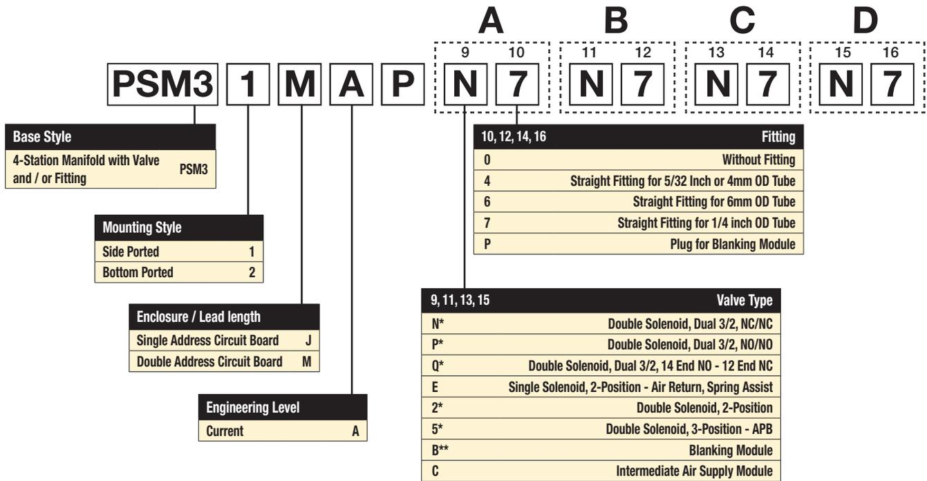
\* Requires double address circuit board, enclosure "M".
