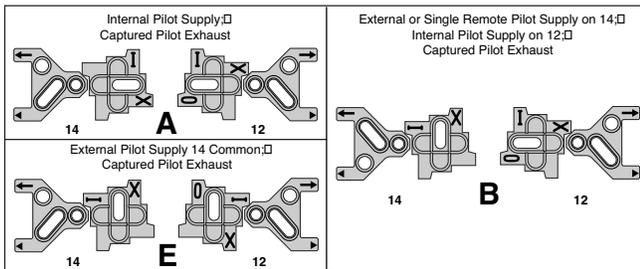
Insert a muffler or vent in the EXH Port of the PEJ02 & PEJ01 Manifold End Plates or #12 of PL02 & PL01 Subbases when using solenoids with **Captured** Pilot Exhaust.
