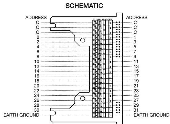
All commons internally connected on terminal strip
