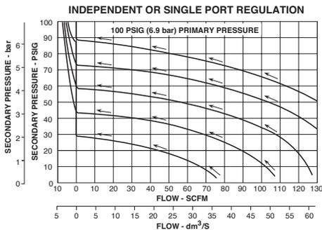
The above curves illustrate flow characteristics through an assembled valve, air regulator, and base (or modular manifold) unit.
