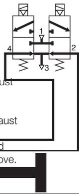
A traditional 5/3 all ports blocked valve is now replaced by a double 3/2 NC+NC valve module and a dual P.O. check module that will block the flow to and from the cylinder. Cylinder positioning is more precise.
