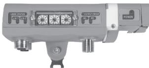
The P2M Industrial Ethernet 24 DO Node offers local diagnostics through 7 LED's located on the visible top side, showing:
