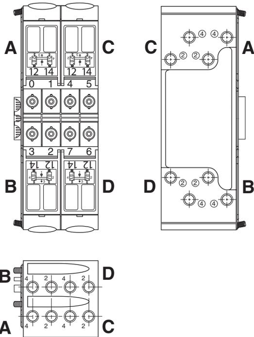
**Double Solenoid - Double Address Manifolds**
