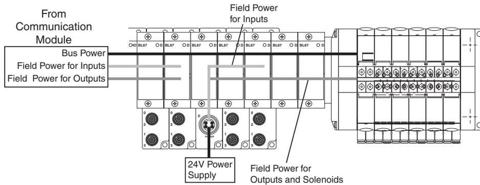
**24VDC Power Extender Module (BL67-PF-24VDC) with Base Module BL67-B-1RSM-VO**
