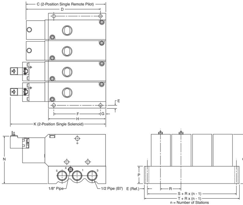
**B7 & B8 3-Way IEM Aluminum Bar Manifold**
