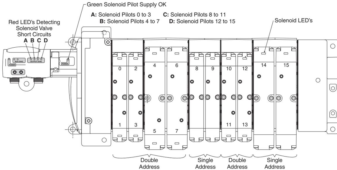
Inside the communication module, solenoid valve control is protected against short-circuits with the following visual indication provided:
