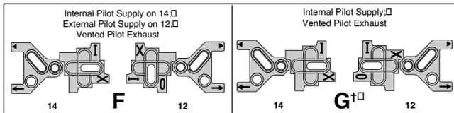
† A plug may be inserted in the EXH Port of the PEJ02 & PEJ01 Manifold End Plates or #12 of PL02 & PL01 Subbases.
