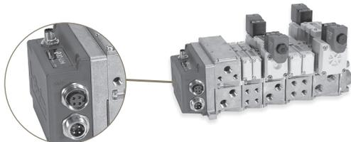
The Class A node has (1) 3 pin M12 connector for communication and logic power from any class A IO-Link master, and (2) 7/8" connectors for auxiliary valve power IN and OUT.
