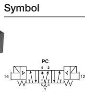
B5 shown, 3-Pin DIN 43650C electrical connection. Non-locking flush override.
