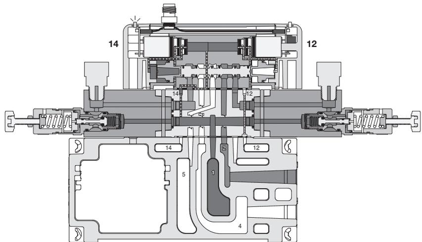
*When using an Independent Pressure Sandwich Regulator, the cylinder outlet ports are reversed. The 12 end energizes the #4 port and the 14 end energizes the #2 port. The 3-Position CE and PC functions are also reversed. (See schematics on above.)*
