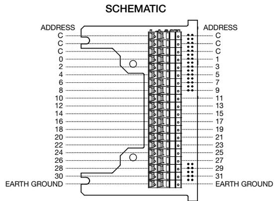
All commons internally connected on terminal strip
