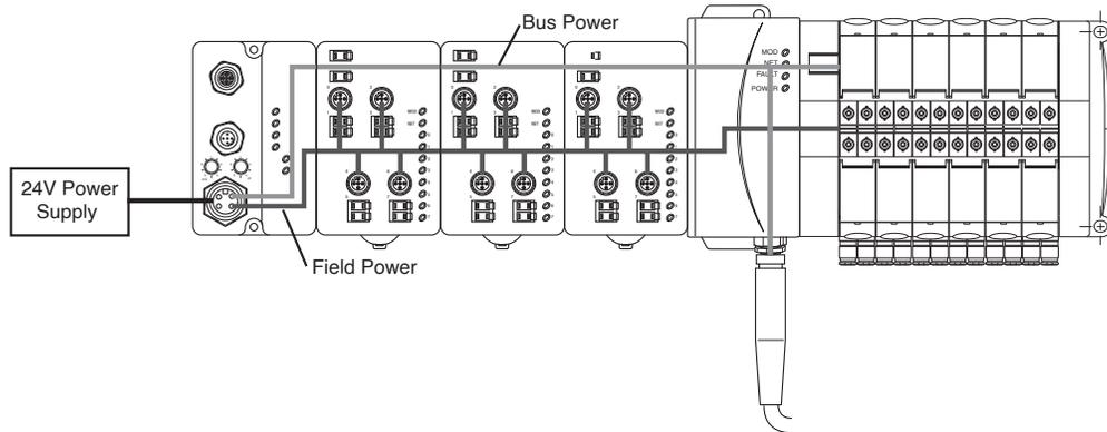
**H Series Network Communication Module with 24VDC and Bus Extension Connectors and I/O Modules**
