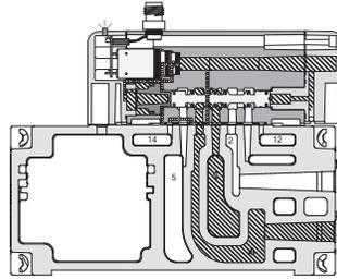
**15407-1** 18mm Single Solenoid Internal Pilot Manifold Mounted
