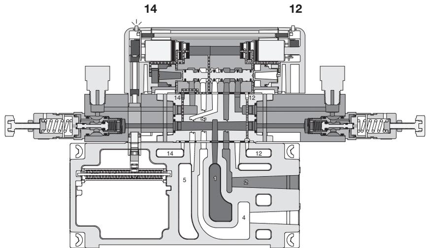
*When using an Independent Pressure Sandwich Regulator, the cylinder outlet ports are reversed. The 12 end energizes the #4 port and the 14 end energizes the #2 port. The 3-Position CE and PC functions are also reversed. (See schematics above.)*
