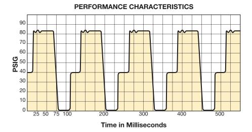
Actual test results show rapid response on a robot welding operation at a major U.S. automotive manufacturer.
