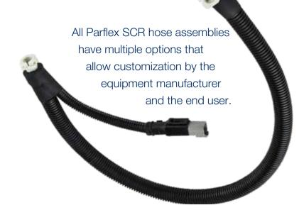
Series SCR - DEF Transfer Hose Visit the webpage Core Tube I.D. With Heat /Abrasion Bend Maximum Vacuum Material Shield Resistance Radius Operating (optional) Pressure mm inch mm inch mm inch psi bar inch/Hg bar mm inch 4.0 .157 14.5 .571 21.0 .827 174 12.0 14.8 500 30.0 1-3/16 **FPDM** 5.5 .217 14.5 .571 21.0 .827 174 12.0 14.8 500 40.0 1-9/16
