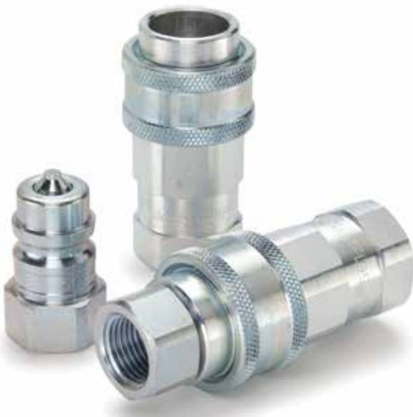
SM Series double shut-off couplings are versatile for use across a spectrum of hydraulic applications where fluid lines require connection and disconnection. Couplers and nipples are steel with nitrile seals and are available in 1/4 through 3/4 inch sizes.
