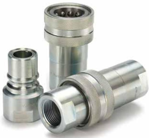
HP Series double shut-off couplings are designed for pressures up to 5000 psi. Couplers and nipples are steel with nitrile seals and are available in 1 and 1-1/2 inch sizes.
