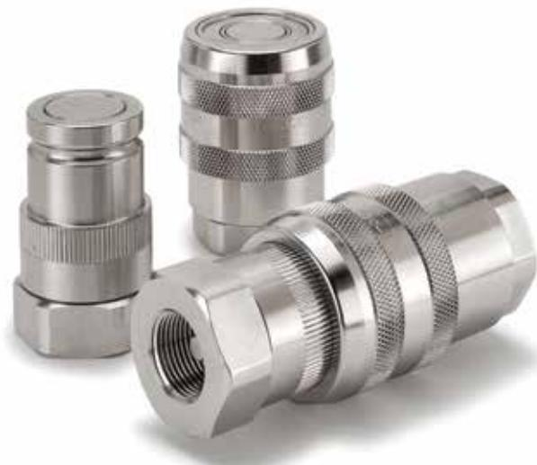
Parker's 71 Series, formerly Snap-tite couplings are designed for working pressures up to 10,000 psi. Available in a variety of materials and with a wide range of body sizes. Air inclusion and fluid loss are minimal with the flush face valves. Large flow chambers in the body and an exclusive valve design permit superior flow while maintaining low pressure drop.
