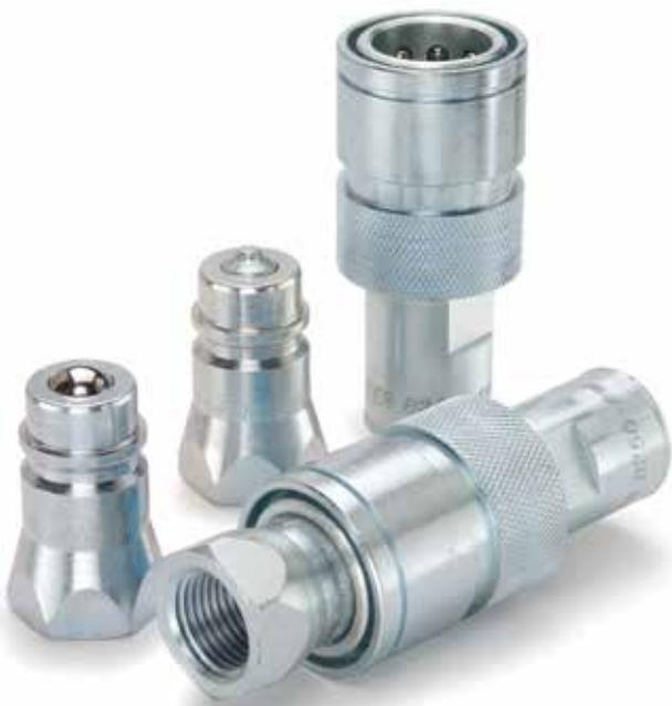
Parker's 8200 Series unique valve design allows connection while either or both the coupler and nipple are under pressure. Valves in both halves remain closed, opening only when system pressure has been relieved on the female body and then reapplied. This pressure sequence may be done with either an open center or a closed center hydraulic system that has a control valve.
