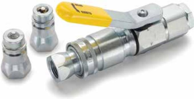
The 9200 Series coupler allows zero pressure connection and disconnection while either or both the coupler and nipple are under pressure. A lever operated cam locks both coupler and nipple valves in the open or closed position. "Closed", the flow is shut off at the coupler, allowing easy connect and disconnect. Valves in the "Open" position are locked in place and unaffected by hydraulic surges. Valves will automatically close if the coupling is accidentally disconnected.
