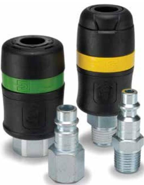
Tool-Mate Series are light weight and easy to operate with a non-marring body. Exhaust style couplers allow disconnection at zero pressure to avoid dangerous hose whip. Couplers are constructed of Polyamide material with galvanized steel port ends. Springs, balls and pins are stainless steel and locking fingers are polyacetate. Black body color designates venting, exhaust style coupler.
