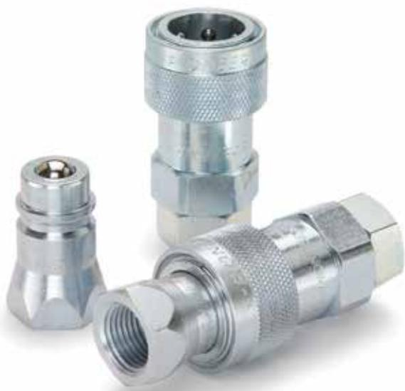
The 5000 Series is an economical coupling that can be connected under pressure where tools can be used to make the connection. The coupler and nipple are connected and then the valves are opened from tightening the threaded union on the back of the coupler body. Unscrewing the body threads will permit the valves to close and the coupler sleeve can be retracted to release the nipple.
