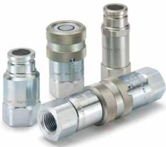
FF Series couplings eliminate spillage and air inclusion when connecting and disconnecting. The sleeve locking mechanism prevents accidental disconnection. 3/8" body size complies with Hydraulic Tool Manufacturers Association standards. FC nipples provide a connect-under-pressure option for trapped pressures up to 3000 psi on the nipple side.
