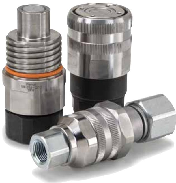
59 Series couplings are ideal for use in high pressure, high impulse applications that require the security of a threaded connection and the ability to connect and disconnect under pressure. The robust ACME thread has a double start and allows full connection to be quickly completed in 2-1/2 turns. An internal bearing between the collar and the body keeps resistance to a minimum for an easy connection.
