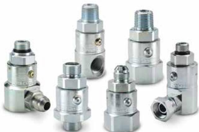
The PS Series Swivel is designed to meet today's application needs and performance requirements. Pressure capabilities up to 5000 psi, 3/8" through 1" body sizes, a variety of port options, and Chromium-6 Free plating make the PS Series Swivels ideal for an array of dynamic applications.
