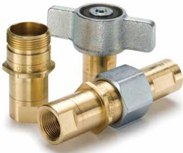
6100 Series is a thread to connect, low spill coupling that can be connected under pressure. Coupler and nipple bodies are corrosion resistant brass. Couplers are available with a steel hex nut or heavy duty wing nut sleeve. A connection indicator groove on the nipple body indicates when the connection is complete and the valves are fully open.
