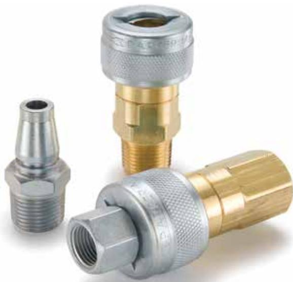
TL Series Pneumatic Couplers are interchangeable with Schraders Twist-Lock style couplings. Couplers have brass bodies and steel sleeves. Nipples are constructed of steel.
