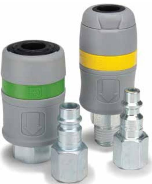
Tool-Mate Series are light weight and easy to operate with a non-marring body. Couplers are constructed of Polyamide material with galvanized steel port ends. Springs, balls and pins are stainless steel and locking fingers are polyacetate. Grey body color designates standard, non-venting style coupler.
