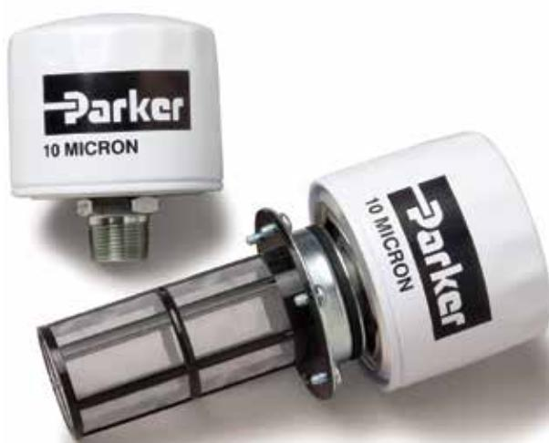
PV Series is an economical Pressure/Vacuum Relief Valve used to maintain positive pressure in hydraulic reservoirs. The large filter area makes this valve an ideal choice for use in heavily contaminated environments. The optional bayonet type mount allows the valve to be installed in the tank filler port, eliminating the need for an extra port. In this configuration, the valve also serves as a filler cap.
