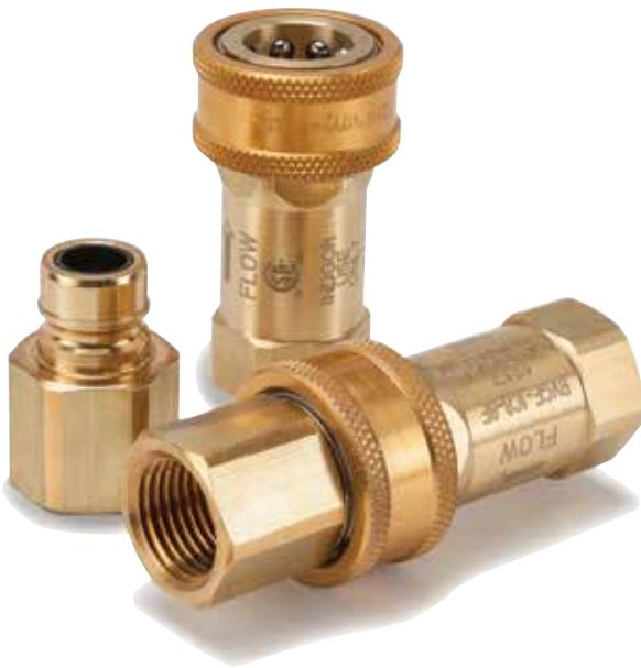
GF/GF-1 Series couplings are valved on the coupler half and will automatically shut off gas flow when coupling is disconnected and automatically open on connection. They also incorporate a safety fuse in the nipple that will shut off the gas supply to your application in the event temperatures exceed 350°F.
