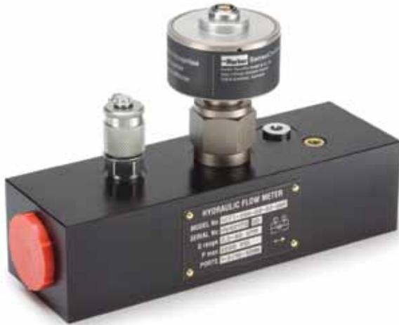
Parker Flow Sensors provide the ability to measure pressure, temperature and flow from a single test point in a hydraulic system. Constructed of light-weight aluminum, they are designed to be used with a wide variety of hydraulic fluids. This design also minimizes the effect of viscosity changes.
