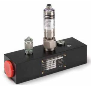
Parker Flow Sensors provide the ability to measure pressure, temperature and flow from a single test point in a hydraulic system. Constructed of light-weight aluminum, they are designed to be used with a wide variety of hydraulic fluids. This design also minimizes the effect of viscosity changes.
