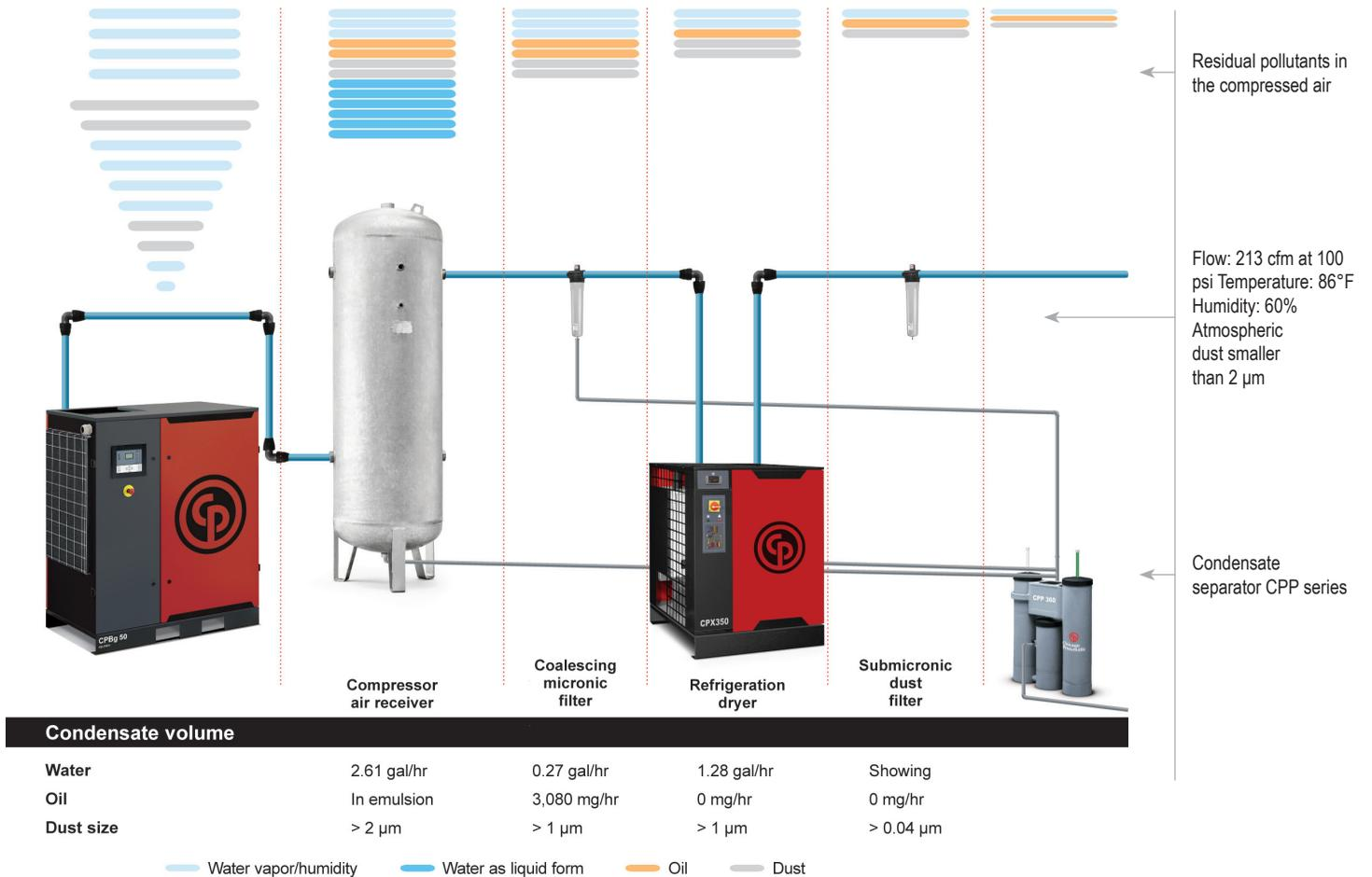
This drawing illustrates that during the air treatment process, 4.16 gallons of water per hour, plus dust, and 3,080 mg/hr of oil are produced. The CPP Condensate Separator will reduce this oil content to 4 mg/gal. With such a small residual amount, it is possible to discharge the condensate, with no risk to the environment.
