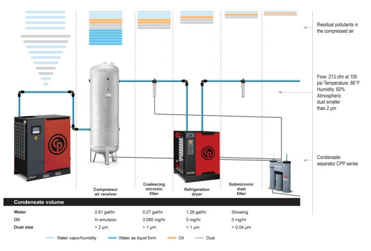
This drawing illustrates that during the air treatment process, 4.16 gallons of water per hour, plus dust, and 3,080 mg/hr of oil are produced. The CPP Condensate Separator will reduce this oil content to 4 mg/gal. With such a small residual amount, it is possible to discharge the condensate, with no risk to the environment.
