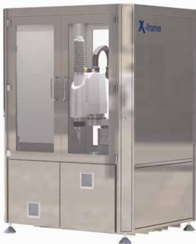
Fig.: Cleanroom cell with cables, installed in the X-frame rack
