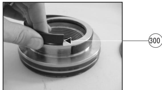
**5.** Install the exclusion seal (207) onto the end cap (4).
