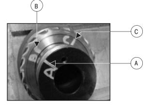
**12.**Remove the O-ring (211) and the backup ring (212) from the end cap (4).
