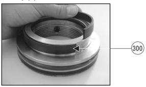
**15.**Remove the main pressure seal (208).
