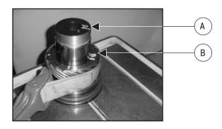
**3.** If applicable, slide the stop tube (400) over the shaft.
