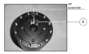
**5.** Using a hex wrench, remove the set screws (106) and steel balls (118) from the end cap.
