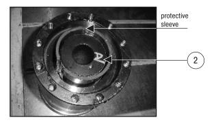
8. Place a round wooden block or round metal plate on top of the protective sleeve, apply even pressure from a drill press, or gently tap evenly with a rubber mallet, until the shaft gently disengages from the housing. Lift the housing up and away from the shaft.
