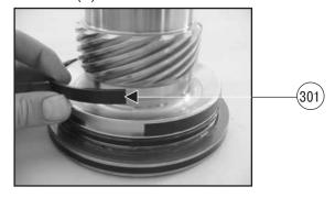
**18.**Remove the main pressure seal (209).
