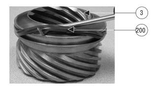
**22.**Remove the piston sleeve (3) ID seal (202) using a small pick or seal tool.
