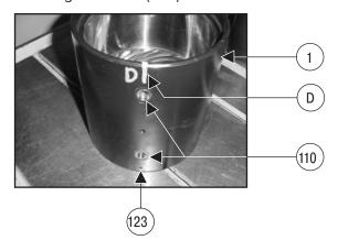
**6.** Make a timing mark (E) with a marker, in line with the female grease zerk (item 123 on assembly drawing page 7) on the shaft flange (2).
