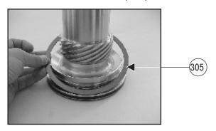
**20.**Remove the exclusion seal (210), from the shaft (02).
