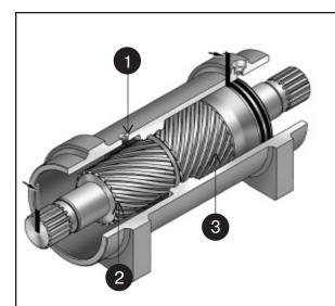
Bars indicate starting positions of piston and shaft. Arrows indicate direction they will rotate. The housing with integral ring gear remains stationary. For clarity, the shaft flange, bearings, and end cap are not shown.
