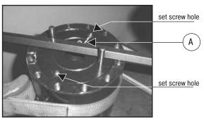
14. Visually inspect each locking hole in the end cap (4) for alignment and possible grease and/or debris. Clean as needed. Place the appropriate size steel ball (118) (see spec chart below) into each locking hole. Using the proper size hex wrench, insert a set screw (106) coated with Loctite 242 locking compound into each locking hole, securing the end cap to the shaft.
