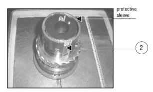
**5.** Make a timing mark (D) on the top lip of the housing (1), directly in line with the two hydraulic ports (110) on the side with the female grease zerk (123).
