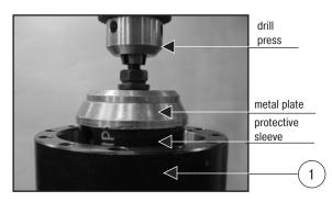
9. Insert two cap screws into the shaft flange (02) and secure to slotted table with threads facing up. Place a strap wrench around the piston (03) gear teeth, turn clockwise until the piston is seated against the shaft.
