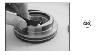
**5.** Install the exclusion seal (207) onto the end cap (4).
