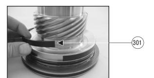
7. Install the wear guide (300) onto the end cap (4).
