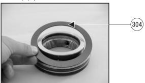
**14.** Remove the wear guide (300) from the end cap (4).
