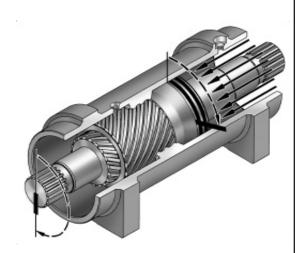
Applying fluid pressure will displace the piston axially while the helical gearing causes the piston and shaft to rotate simultaneously. The double helix design compounds rotation: shaft rotation is about twice that of the piston. Applying pressure to the opposite port will return the piston and shaft to their original starting positions.
