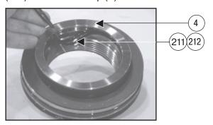
**13.**Remove the thrust washer (304) from the end cap (4)
