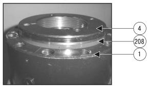
13. Insert pins into the end cap (4) spanner holes. Using a pry bar, screw the end cap on by turning it in a clockwise direction until it becomes tight (see General Torque Guidelines chart). Use the reference mark (A) made during the disassembly process, as a reference point to line up the two set screw holes in the end cap with the grind marks (dimples) on the shaft threads.
