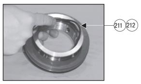
**10.**Install the piston sleeve ID seal (202) into the piston (3) using a circular motion.
