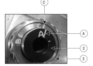
2. Place a strap wrench around the piston OD (3) gear teeth, rotate the piston clockwise. The piston will engage the shaft (2) gear teeth. Rotate piston until it is firmly seated against the shaft
