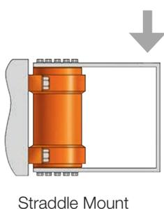
The upper portion of the bracket is bolted to the shaft flange, the lower portion is bolted to the endcap flange.
