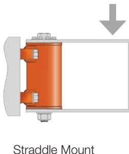
The upper portion of the bracket is bolted to the shaft flange. The lower portion is secured either by a tie rod passed through the shaft bore or is bolted to the endcap flange.
