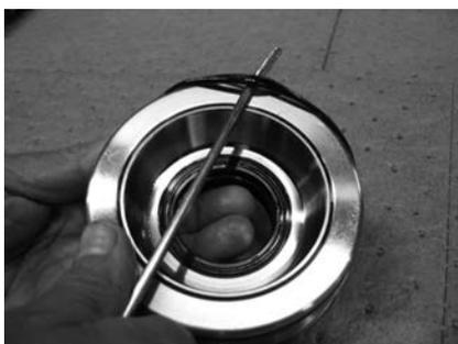
3. Remove end cap I.D. wiper seal (206).
