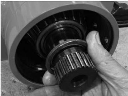
9. Remove the bearing (108). Take note of which end the bearings are removed, so they can be paired with the same bearing race during
