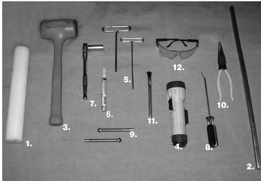
Several basic tools are required for the disassembly and reassembly of the actuator. The suggested tools are outlined below:
