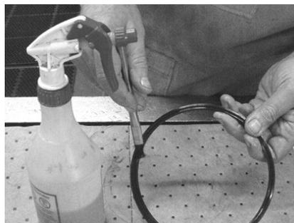
3. First, install the end cap O.D. B/U ring seal (209.2) to the end cap (04). Ensure the concave side of the B/U seal faces the O-Ring.
