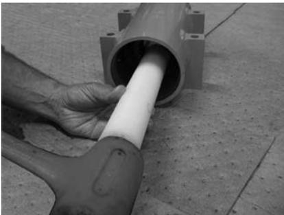
3. Place a mark on the housing (01), and on the piston sleeve (03) in line with a port fitting or some other reference. This will simplify the process of aligning the piston to the ring gear teeth during re-assembly.
