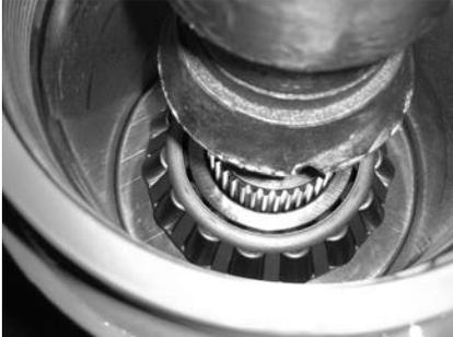
3. Remove bearing from the shaft. Verify timing marks on the shaft.
