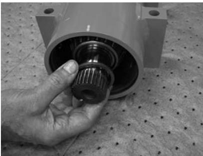
**NOTICE** It may be necessary to heat T20-60 bearings to 200° Fahrenheit prior to installing on each end of the shaft for a slip fit.
