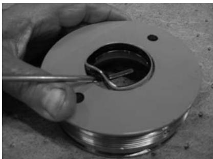
4. Remove the piston sleeve O.D. cup seals (202, 203) from the piston (03).
