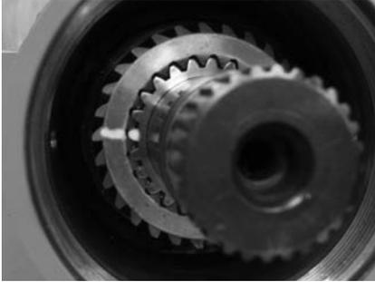
2. Slowly turn the piston sleeve (03) while using a plastic hammer and mandrel to gently tap the piston sleeve (03) to disengage the gear teeth from the housing ring gear teeth inside the housing bore.
