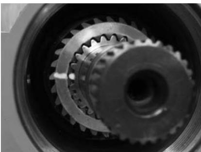
2. Slowly remove the shaft (02) from the piston sleeve (03) by pulling and turning at the same time.
