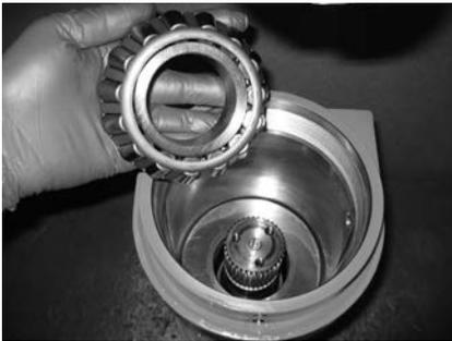
4. Install bearing splitter and replace shaft in the ram.
