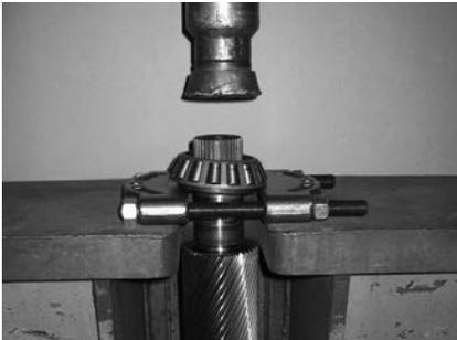
6. Remove bearing from the shaft.
