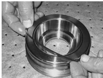
4. Next, install the end cap O.D. O-ring seal (209.1) into the end cap (04). Seal (209.1) is slightly smaller in diameter than (204).
