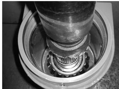
2. Depress ram to force shaft downward to release the bearing.
