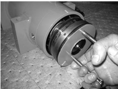
8. Remove the seal (205) and spacer (113).
