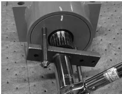
4. For re-drilling actuators with dowel pins (109), use a drill bushing to create a 0.188" diameter hole. Drilled depth should match the dowel pin hole on the opposite end. Do
