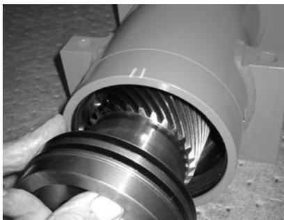
sleeve (03) timing marks with timing marks in the housing (01).
