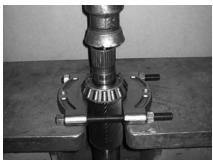
5. Depress ram to force shaft downward to release the bearing.
