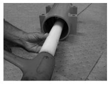
**3**. Place a mark on the housing (01), and on the piston sleeve (03) in line with a port fitting or some other reference. This will simplify the process of aligning the piston to the ring gear teeth during re-assembly.
