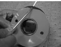
2. Remove end cap O.D. O-ring seal (209.1) and B/U ring seal (209.2).
