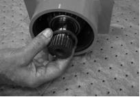
**2**. Coat end cap (04) threads with anti-seize grease.
