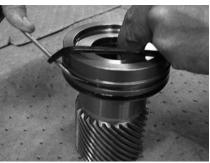
**10**. Remove the energizer from the piston sleeve I.D. cup seal (201) prior to installation. Install the piston sleeve I.D. cup seals (200) and (201) inside the piston sleeve (03). (201) should be closest to the gearing.
