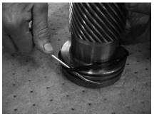
**9**. Install the piston sleeve O.D. cup seal (202) onto the piston sleeve (03). (This seal should still have the energizer in it.)
