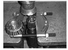
Check the condition of the bearings after the removal procedure, they may need to be replaced.
