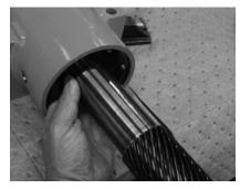
**3.** Verify the timing marks before fully rotating the shaft into the piston sleeve (03).
