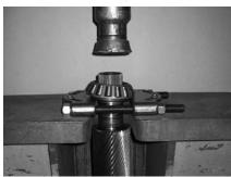
6. Remove bearing from the shaft.
