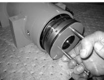
8. Remove the seal (205) and spacer (113).
