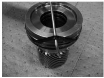
5. Remove the piston sleeve I.D. cup seals (200, 201) from the piston (03).
