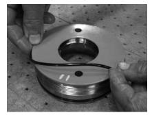
6. Install the end cap I.D. wiper seal (206) into the end cap (04).
