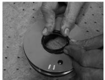
If needed remove the energizer (small O-ring) from the inside the piston sleeve O.D. cup seal (203) prior to installation. Also remove the energizer from inside the piston sleeve I.D. cup seal (201).
