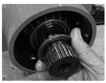
**9**. Remove the bearing (108). Take note of which end the bearings are removed, so they can
