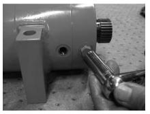
**4**. Use the needle nose plier to remove the dowel pin that locks the end cap.
