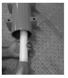
until the front of the piston sleeve (03) is lined up with the timing marks on the housing (01) ring gear.
