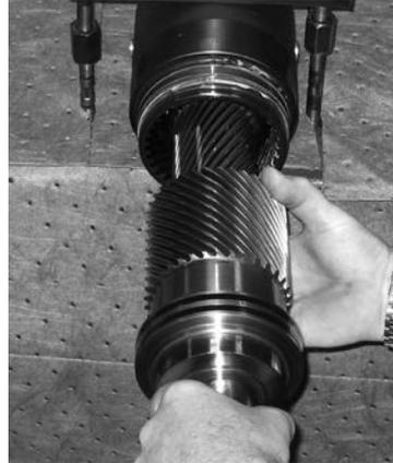
2. Look inside the housing. Timing marks (center punches) will be visible on the ring gear inside the housing and the piston sleeve. Typically there should be two marks close together on the piston sleeve one for the inside and outside gear teeth. If no timing marks are located on any items, use a push type center punch to make new marks.
