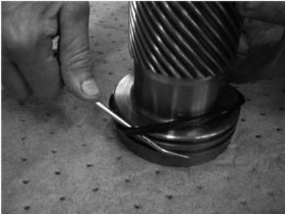
7. Install the piston sleeve O.D. cup seal (203) onto the piston sleeve (03). Make sure to remove the energizer from the cup seal to prevent pressure trapping.
