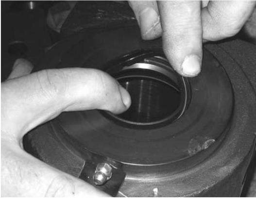
3. Install O-Ring (230) then O-Ring (220) and B/U Ring (221) onto P1 (01.1) housing half.
