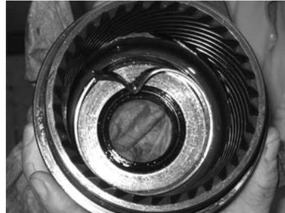
4. The bushing in the P1 housing half is accessible only through the inside of the housing. Using a chisel punch, carefully collapse the bushing enough to relieve the press fit. Care must be exercised to prevent damage to the housing.
