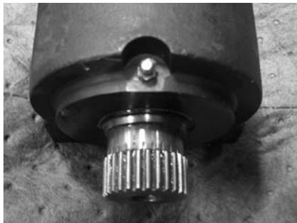
3. Firmly secure the P1 (01.1) end of the actuator housing to a work bench.
