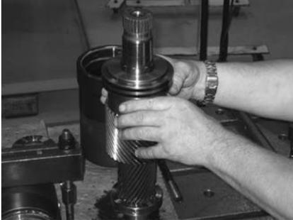
3. Press the bearing retainer (05) onto the P2 end of shaft.
