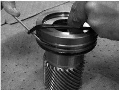
8. Remove and discard the energizer from the piston sleeve I.D. cup seal (201) prior to installation. Install the piston sleeve I.D. cup seals (200) and (201) inside the piston sleeve (03). (201) should be closest to the gearing.
