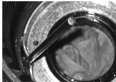
5. Remove the bushing and thrust washer from the P1 housing half.
