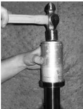
4. Install cup seals (205) onto both ends of piston shaft assembly.
