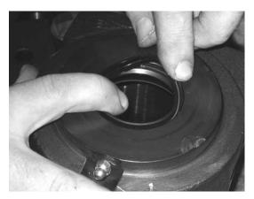
Install O-Ring (230) then O-Ring (220) and B/U Ring (221) onto P1 (01.1) housing half.
