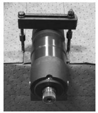
4. Insert 5/8-11 bolts or studs into mounting holes in P2 housing half feet.
