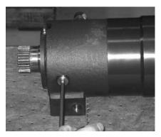
**2**. Remove the grease fittings (111) from each end of the housing.
