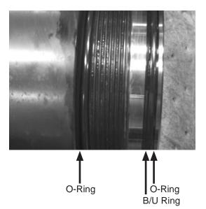
Remove and discard the energizer (small O-Ring) from the inside of the piston sleeve O.D. cup seal (203) prior to installation. Also remove the energizer from inside of the piston sleeve I.D. cup seal (201).
