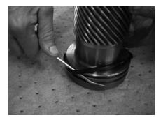
Install the piston sleeve O.D. cup seal (203) onto the piston sleeve (03). Make sure to remove the energizer from the cup seal to prevent pressure trapping.
