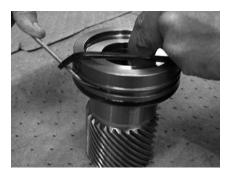
Remove and discard the energizer from the piston sleeve I.D. cup seal (201) prior to installation. Install the piston sleeve I.D. cup seals (200) and (201) inside the piston sleeve (03). (201) should be closest to the gearing.
