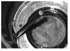
5. Remove the bushing and thrust washer from the P1 housing half.
