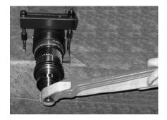
2. Look inside the housing. Timing marks (center punches) will be visible on the ring gear inside the housing and the piston sleeve. Typically there should be two marks close together on the piston sleeve one for the inside and outside gear teeth. If no timing marks are located on any items, use a push type center punch to make new marks.
