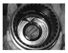
4. The bushing in the P1 housing half is accessible only through the inside of the housing. Using a chisel punch, carefully collapse the bushing enough to relieve the press fit. Care must be exercised to prevent damage to the housing.
