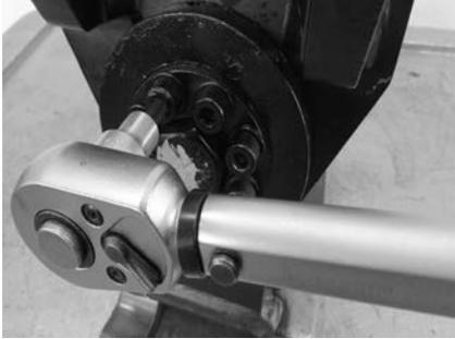
2. Insert screw (409), 1" tie-rod bolt through center of PowerTilt from the torque foot end, install spacer (410) and lock-nut (411) and torque to 920 Nm (680 ft-lbs).
