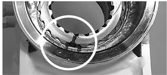
piston sleeve (3). Use a plastic mallet and mandrel if necessary. Avoid scratching or denting the inside of the housing bore.
