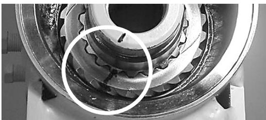
tap the end of the shaft with a plastic mallet and mandrel if needed.
