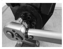
2. Insert screw (409), 1" tie-rod bolt through center of PowerTilt from the torque foot end, install spacer (410) and lock-nut (411) and torque to 920 Nm (680 ft-lbs).
