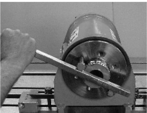
4. Remove the two screws and tighten the end cap (04) using a torque wrench and customized end cap tool to the torque specifications shown on the End Cap Torque Chart on Page 41.
