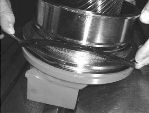
2. Lightly coat both sides of the thrust washer (344) with Lithium grease and install onto the shaft (02).
