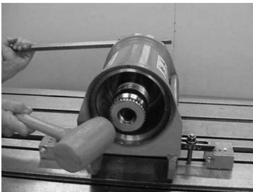
2. Locate the timing marks on the housing ring gear (1.4), piston sleeve assembly (03) and shaft (02). Small punch marks are usually found on the face of the piston teeth and ring gear. The shaft timing marks may be located in the root or "V" of the helical gearing. Piston sleeve timing marks are best seen when the splined end of the piston sleeve is flush with the ring gear inside the housing.
