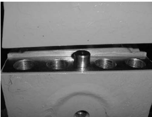
5. Then install the coupler (06) onto the shaft (02). Align the dowel pin (105) on the shaft to the torque foot (6.1).
