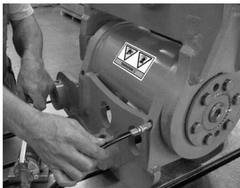
2. Locate the grease fittings (122) or ports on the end of the PowerTilt and using a grease gun, pack the exclusion seal and thrust washer with grease until it exhausts from the grease reliefs (123).
