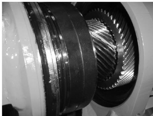
3. Remove the shaft (02) by rotating and sliding the shaft gear teeth out of engagement with the inside diameter gear teeth of the piston sleeve assembly (03).
