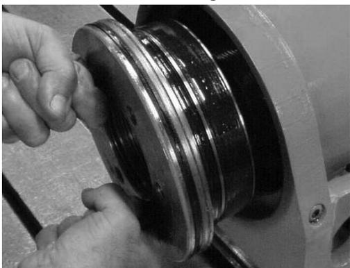
3. Using a pry bar, continue to rotate clockwise and tighten until the thrust washer (344) makes contact with the housing (01) collar.
