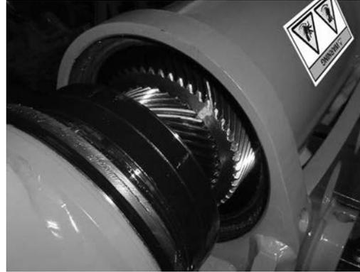
4. Use a pry bar to rotate the shaft (02) in until it is completely bottomed out in the housing (01).
