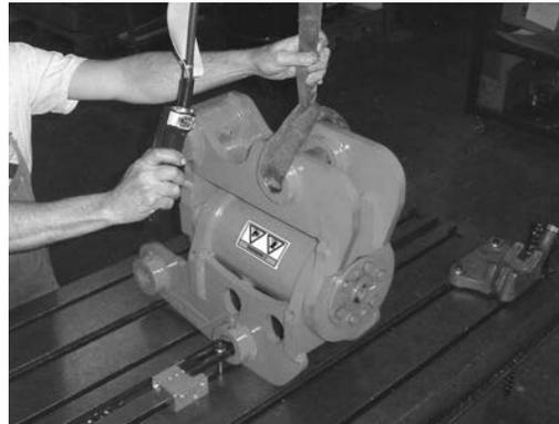
6. Insert threaded bolts into the lock ring (05) and pull straight out.
