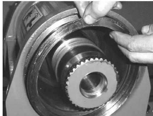
2. Remove the lock ring O-ring (239) from the shaft.
