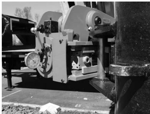
1. Loosen and remove the lock ring bolts.
