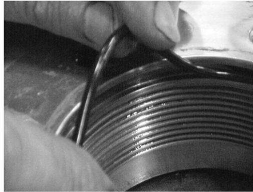
3. Next install the O.D. pressure seal (238) with the lip facing inboard toward the hydraulic pressure.
