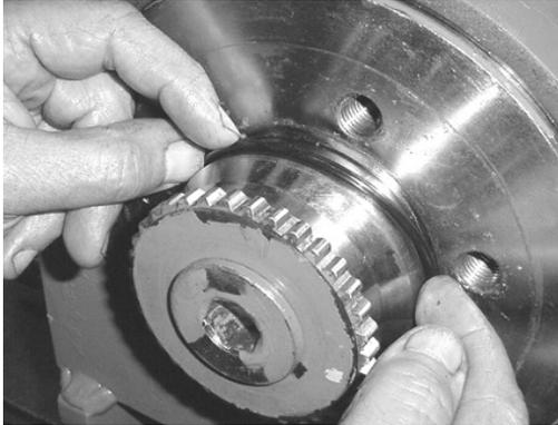
8. Next install the lock ring (05) using two threaded bolts as handles.
