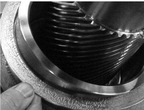
3. Then install the pressure seal (238) with the lip facing inboard, toward the hydraulic pressure.
