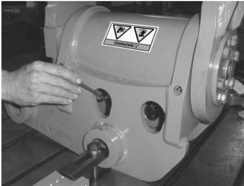
2. When removing the standard pin-on coupler or torque foot (6.1) and idler foot (6.2), remove the shaft mounting screws (104).
