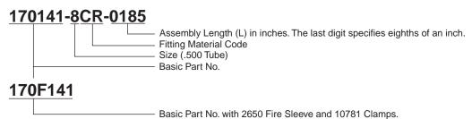
Hose Assemblies with FLARELESS fittings meet the requirements of AS604 (formerly MIL-H-38360) and AS (MS)drawings referenced. Fittings mate with AS4375/MS33514 type connectors. Assembly length measured from **END of nipple to END of nipple**. See "MEASUREMENT OF FLARELESS HOSE ASSEMBLIES" (page 4) to convert to/from GAGE POINT to GAGE POINT assembly length.
