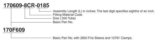
Hose Assemblies with Beam Seal fittings conform to part numbers shown. Fittings mate with AS4207/MIL-F-85421/1 type connectors. Assembly length measured from END of nipple to END of nipple.
