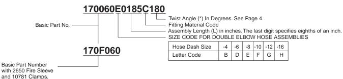
Assembly length measured from END of nipple to END of nipple.
