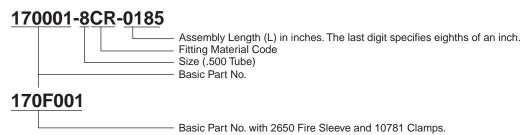
Hose Assemblies with FLARE fittings conform to AS604 (formerly MIL-H-38360) and AS(MS) part numbers shown. Fittings mate with AS4395/MS33656 type connectors. Assembly length measured from END of nipple to END of nipple.
