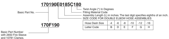
Assembly length measured from **END of nipple to END of nipple**. See "MEASUREMENT OF FLARELESS HOSE ASSEMBLIES" (page 4) to convert to GAGE POINT to GAGE POINT assembly length.
