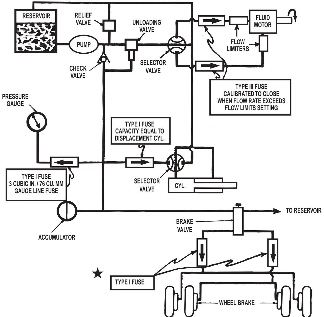
★ FOR SYSTEMS NOT UTILIZING A PRESSURIZED RESERVOIR, THE TYPE II FUSE MIGHT BE BETTER ADAPTED.
