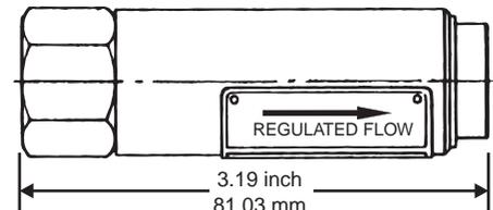
Some flow rates meet requirements of Standard Part Number MS28886, qualified under Specification MIL-V-8566
