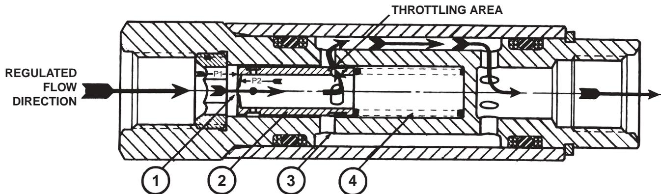
Flow entering the regulator passes through the sharp-edged orifice (1), then flows radially outward through milled slots in the piston (2) and the drilled holes in the body (3). Fluid flows unobstructed through the remaining portion of the regulator to the sub-system.
