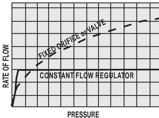
This graphic representation illustrates flow characteristics of the Pressure Compensated Flow Regulator compared with those of a fixed orifice (or restrictor valve).
