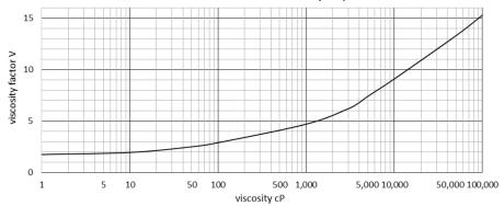
$\begin{aligned} &(\textit{English units}) \, \textit{Total Power} \, (\textit{HP}) = (0.0007 \times p + 0.0051 \times v) \times n \times c \\ &(\textit{Metric units}) \, \textit{Total Power} \, (\textit{Kw}) = \frac{(2 \times p + v) \times n \times c}{1000} \\ &p = \textit{pressure} \, (\textit{psi or bar}) \\ &v = \textit{viscosity correction factor} \, (\textit{from graph}) \\ &n = \textit{speed} \, (\textit{RPM}) \end{aligned}$
