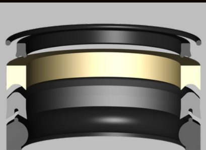
The relationship between the Header Ring and the Pressure Ring
