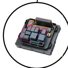
PDM's (aka Power Distribution Modules)
