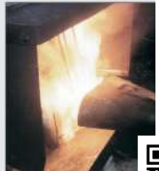
Fire Resistance Testing of Aerospace Hose
